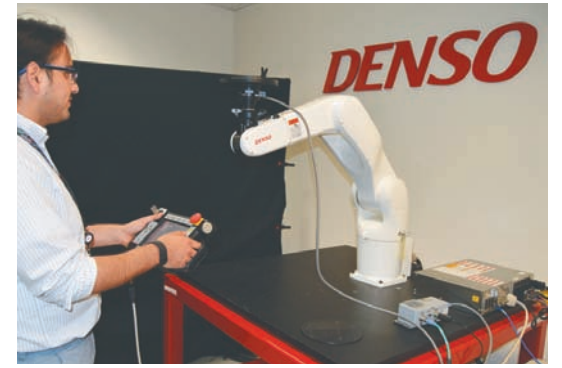
Long Beach-based DENSO Products and Services America Inc. Robotics Engineer Carlos Lopez teaches positions for a DENSO six-axis robot arm integrated with a force/torque sensor. Technology is one of the fastest growing industries in Long Beach. (Photograph by the Business Journal's Larry Duncan)
