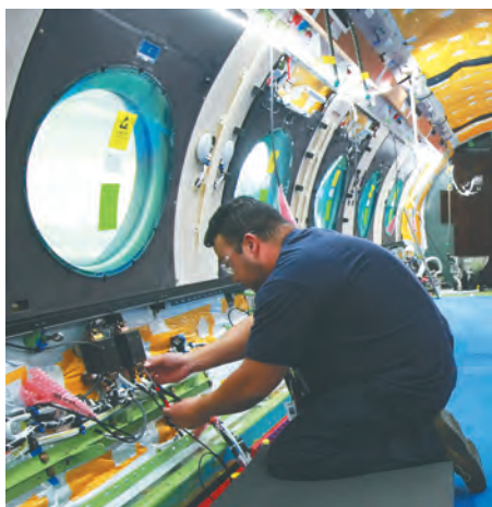
Gulfstream employee Roberto Suncin, an avionics technician, is installing a connector for the Gulfstream Cabin Management System on a G650ER aircraft. The system synchronizes with smartphones and tablets to provide touch-screen control for temperature, lighting, window shades and entertainment options. (Photograph courtesy of Gulfstream)
