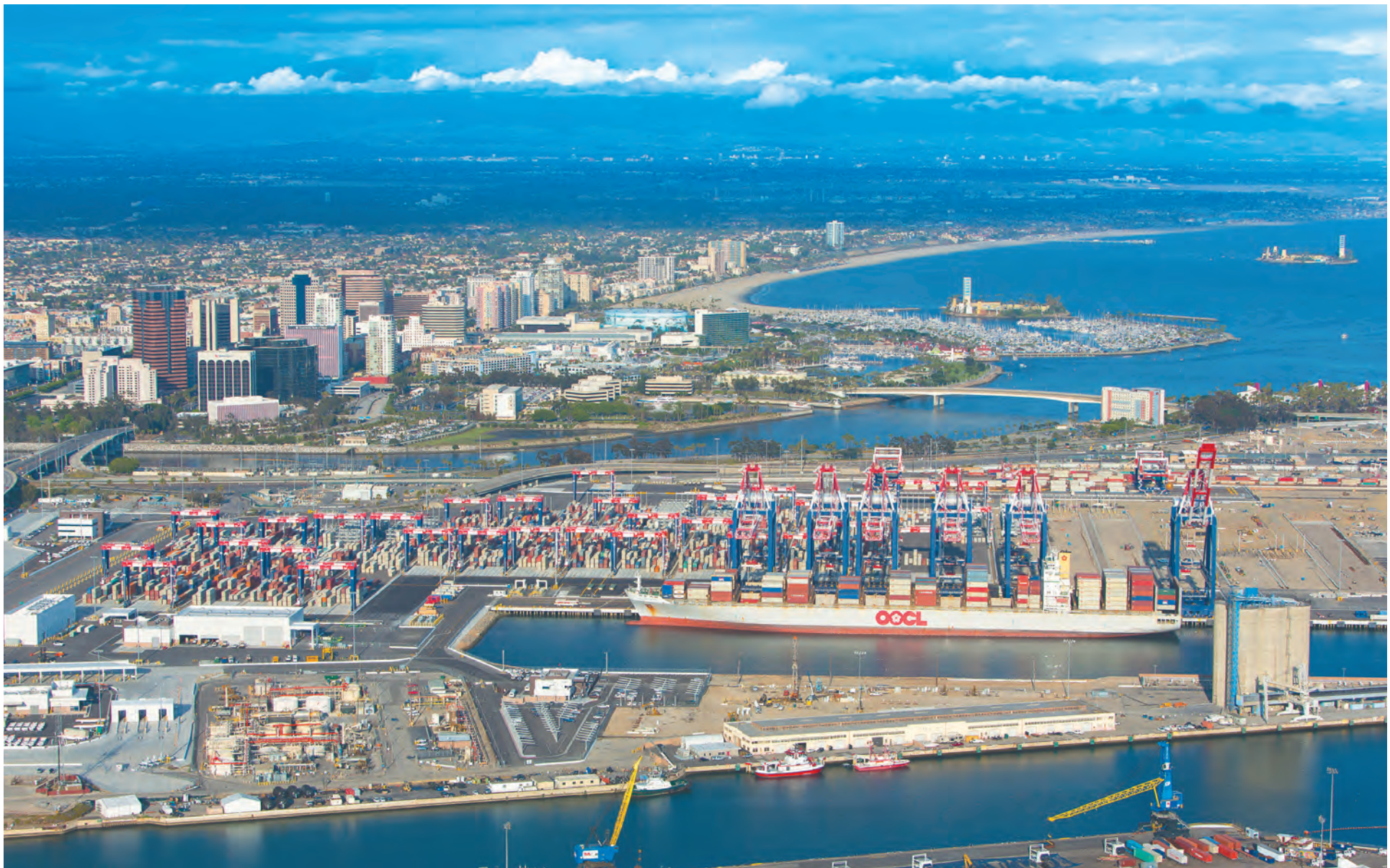
The first phase of the Middle Harbor terminal (center) at the Port of Long Beach was completed last year with the latest technologically advanced cargo handling equipment, including the all-electric stacking cranes, automated guided vehicles (AGVs) and solar panels. The terminal operated by Orient Overseas Container Line's (OOCL) subsidiary Long Beach Container Terminal, Inc. (LBCT) went live this month. The next phase is to be completed in 2019. Pictured in the foreground is a cement terminal. (Port of Long Beach photograph)
