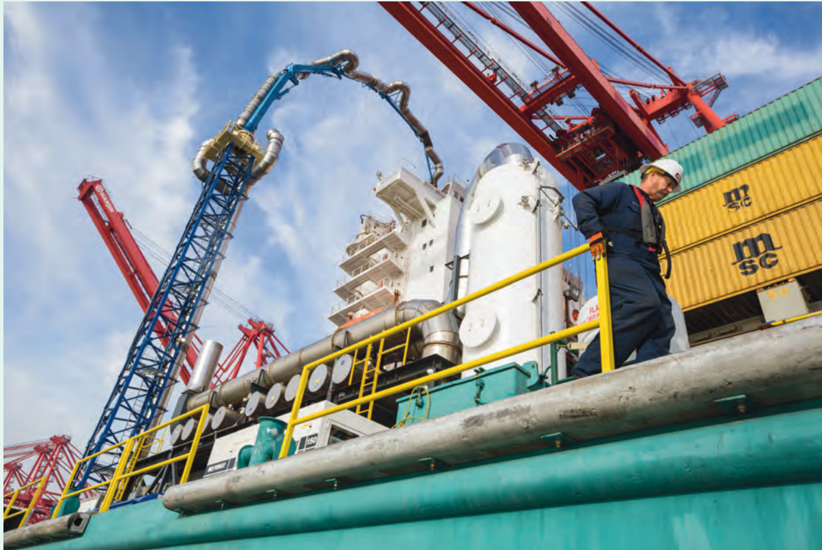
The barge-mounted Advanced Maritime Emissions Control System hooks up to a ship's engine, sucks out harmful air emissions, and cleans the exhaust. The Port of Long Beach has invested in the testing of this equipment, which was recently approved for use on some container ships. (Photograph courtesy of the Port of Long Beach)
