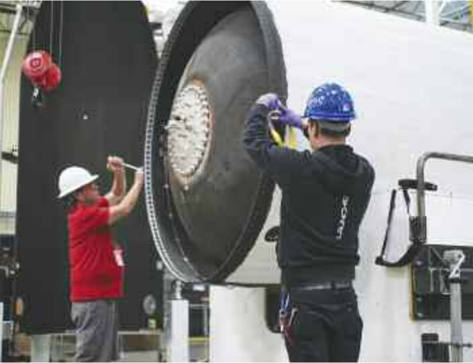
Virgin Orbit technicians work on the first stage of a LauncherOne rocket. The bottom of a fuel tank can be seen inside the rocket’s casing. (Photograph courtesy of Virgin Orbit)
