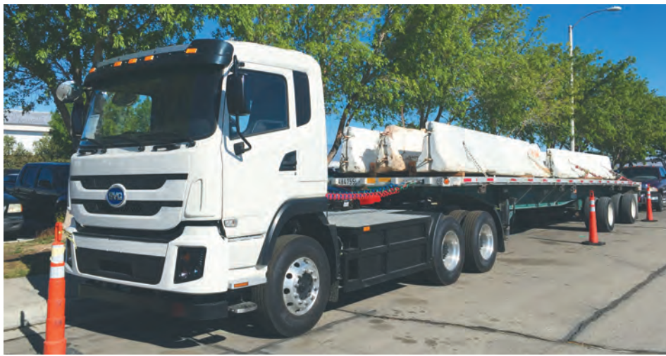
BYD offers an electric, zero-emission heavy duty truck capable of handling payloads similar to those of traditionally-fueled trucks calling the port. BYD's truck only has a range of about 100 miles, but the company is working on another model that would double this range. (Photograph provided by BYD)
