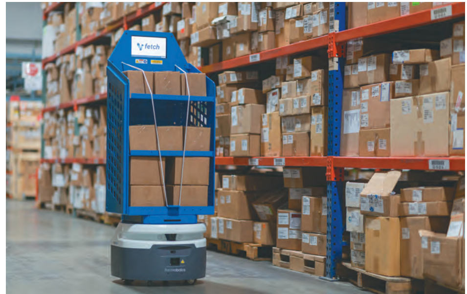
A Fetch Robotics VirtualConveyor™ robot is pictured transferring packaged goods in a warehouse. According to Tim Smith, a representative for San Jose-based Fetch Robotics, their autonomous mobile robots are able to move in a number of directions to transport materials, rather than on a fixed path. (Photograph courtesy of Fetch Robotics)
