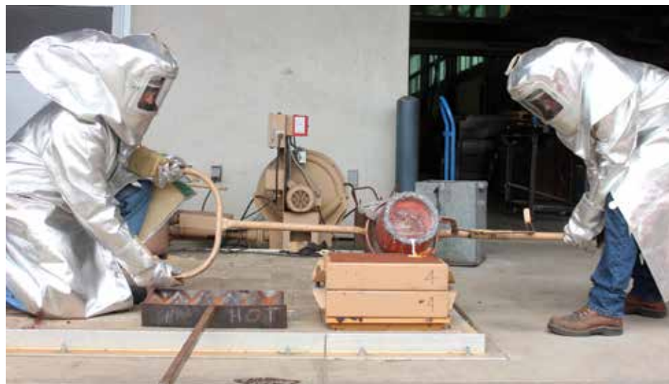
A Long Beach City College instructor and assistant pour molten aluminum into a mold during a metal fabrication class at the Pacific Coast Campus. (Photograph by Brandon Richardson)
