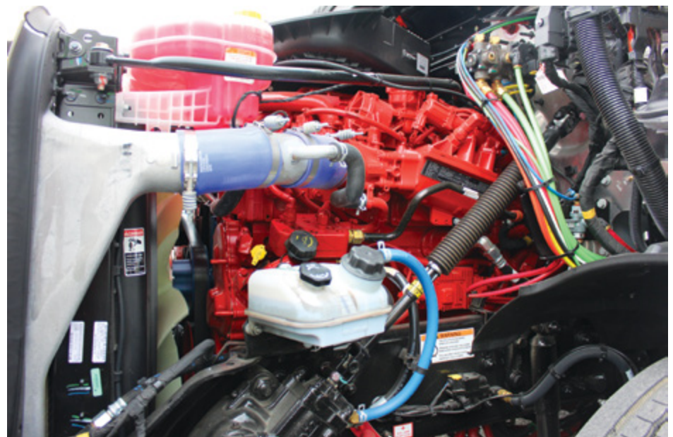
The engines of some near-zero emissions trucks, such as the ones recently acquired by Total Transportation Services, Inc. (TTSI), are powered by renewable natural gas. (Photograph by Brandon Richardson)
