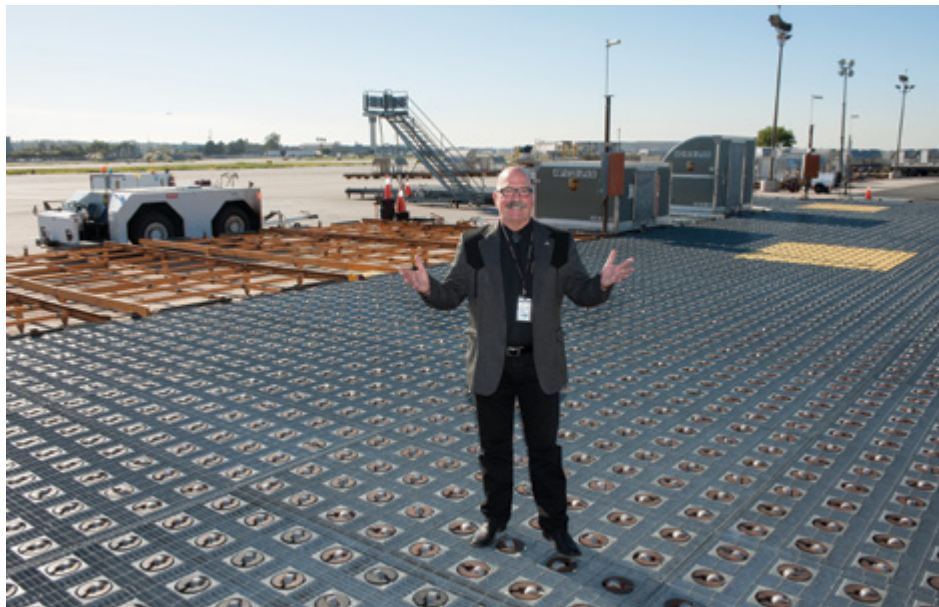
Bruce MacRae, United Parcel Service's vice president of state government affairs for the Western Region, is pictured standing on a caster deck, which is used to sort igloo-shaped "pods" containing air cargo before they are loaded onto a cargo plane. (Photograph courtesy of the Long Beach Area Chamber of Commerce)
