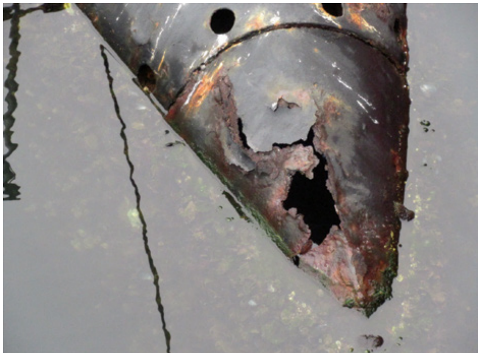
A photograph from the June 2019 inspection report of the Queen Mary property by an independent contractor, Edward Pribronic, shows a hole in the Scorpion submarine. The heavily corroded sub is docked beside the Queen Mary, and in danger of listing or sinking, according to the report. (Photograph courtesy of the City of Long Beach)
