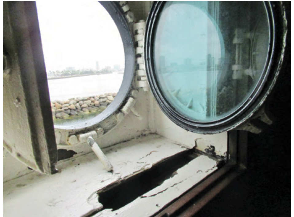
A porthole in view of the public on the Queen Mary languishes in disrepair, as evidenced in this image from a May 2019 by Edward Pribonic, an independent inspector hired by the City of Long Beach to keep track of ship maintenance. (Photograph courtesy of the City of Long Beach)
