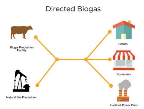
The term "directed biogas" describes the purchase of biogas from a remote production facility, which is then fed into the general gas pipeline accessed by end users, such as the hydrogen fuel cell plant currently in development at the Port of Long Beach. (Infographic by Alena Maschke)
