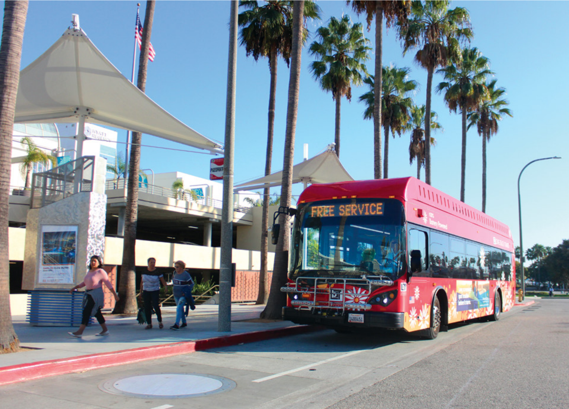
The Passport route, where Long Beach’s first fleet of electric buses premiered, features a Wireless Advanced Vehicle Electrification (WAVE) port set in the pavement, allowing buses to up their charge without docking, if necessary. (Photograph by Brandon Richardson)
